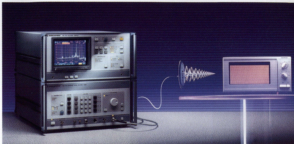
FIG 2 Rohde & Schwarz EMI Test Receiver ESM1 for 20 Hz to 26.5 GHz Photo 40 639
