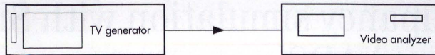
FIG 5 Checking Video Analyzer UAF with predistorted signals from TV Generator SAF or SFF
